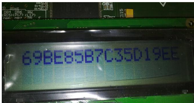
Fig. 4: FPGA implementation of DES Encryption on Spartan 3E kit
